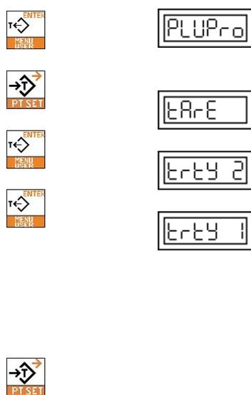
1. Keep pressed the key for longer than 1 second to access the User’s Programming.
