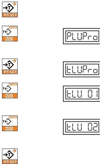
1. In normal working mode, place the tare weight on the platform and press
