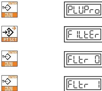
1. Keep pressed the key for longer than 1 second to access the User's Programming
